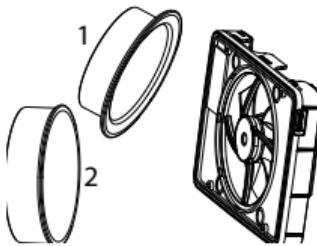
When installing the fan, check that there is a seal between the pipe/duct and wall/ceiling to prevent humid air from penetrating the wall or ceiling. Use the accompanying screw and plug, if necessary.
